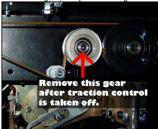
Figure 5 – Slide Gear off Shaft of 2 nd Pinch Roller
