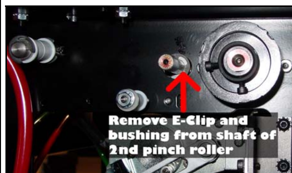
Figure 6 – Remove E-Clip and Bushing from Shaft
