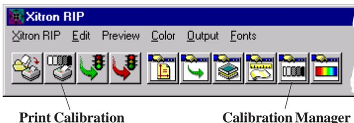
**Calibration (Dot Gain) Manager** displays calibration sets grouped by device. When you select from the **Device** drop-down list, all of the existing calibration sets for that device are displayed. The basic calibration steps are as follows (see the RIP manual for detailed procedures):
