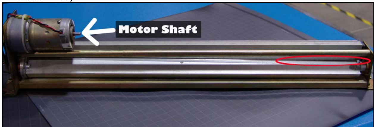
Figure 6 – Blade should fully close gap to cut through whole plate
